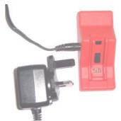
The CanReset is available in two types. One type works from a USB power source whilst the other works with mains electricity.
